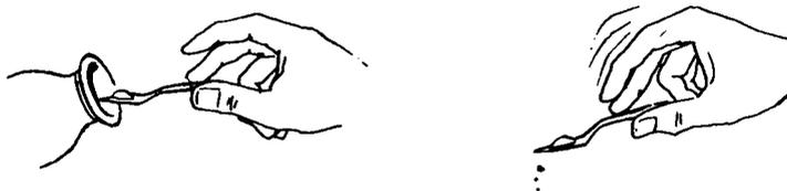
To transfer a chemical from a bottle to a small jar or beaker, remove the stopper from the bottle, tip the bottle and rotate it over the desired container until the proper amount is in the new container.
