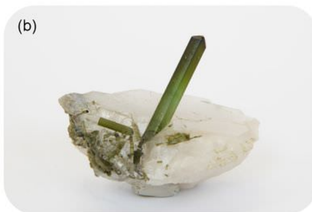
(b) The silica tetrahedra in tourmaline are in rings to create elongated prisms.
